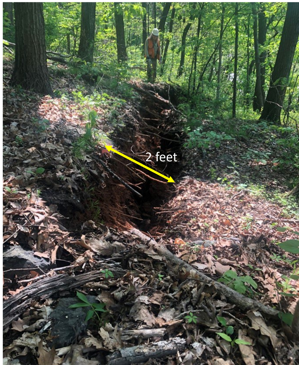
Large tension crack to east of main slide
